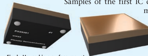
Fig. b: Housed in a surface mount package for PCB assembly, the PS25201 EPIC sensor will be available in this quarter.
